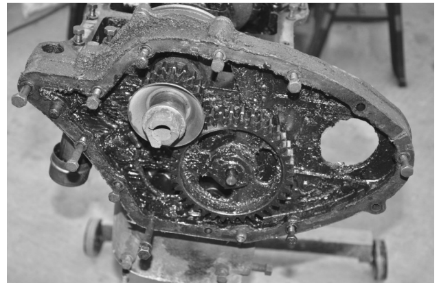
A few years of sludge build-up
